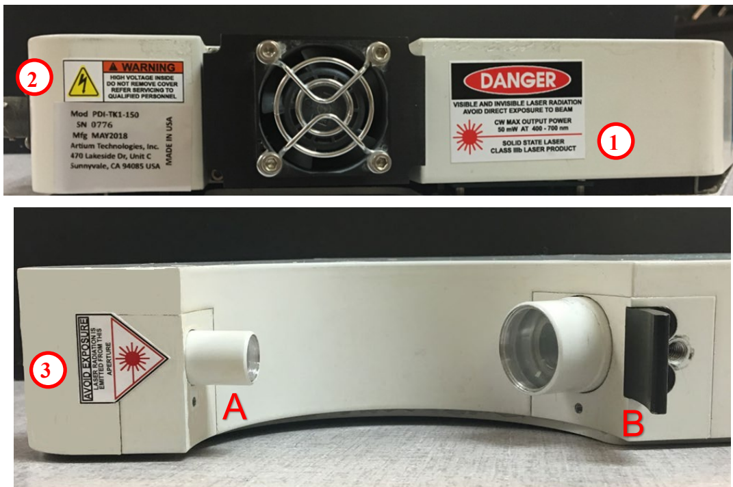
Figure 6.1: Laser beams exit window A and are stopped by beam block B.
