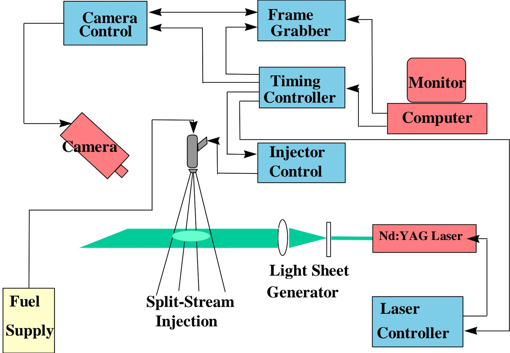
*First Planar Optical Patternator developed for fuel injector spray characterization, S.V. Sankar and W.D. Bachalo 1994.*
