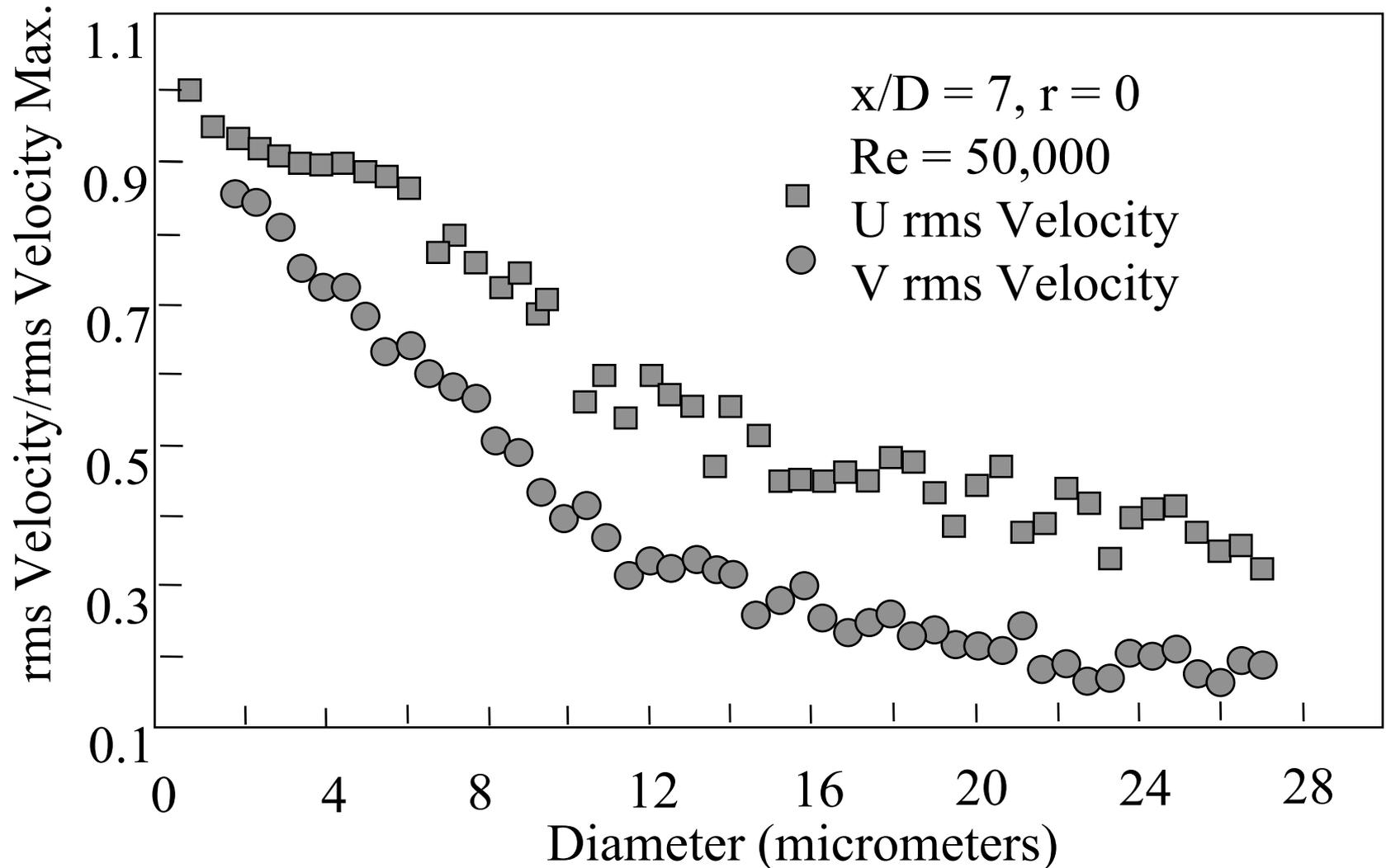
*First measurements of particle response in a turbulent spray flow, S.V.*
