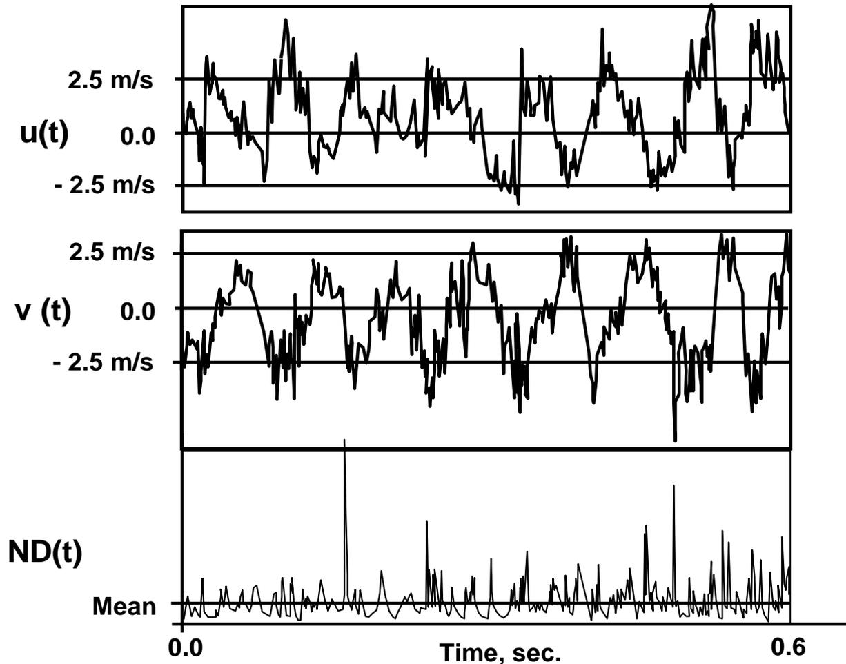
*First measurements of time-dependant behavior of sprays in a turbulent flow, W.D. Bachalo, R. Rudoff, and S.V. Sankar 1988.*
