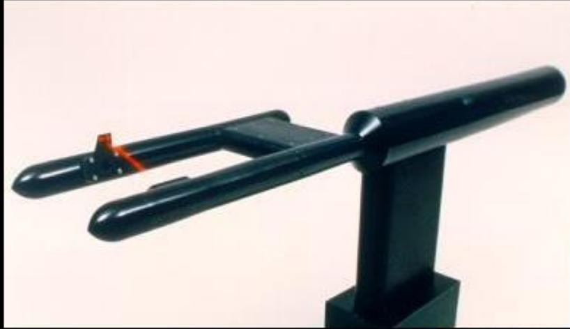
*First PDPA Flight Probe for Aircraft Icing
