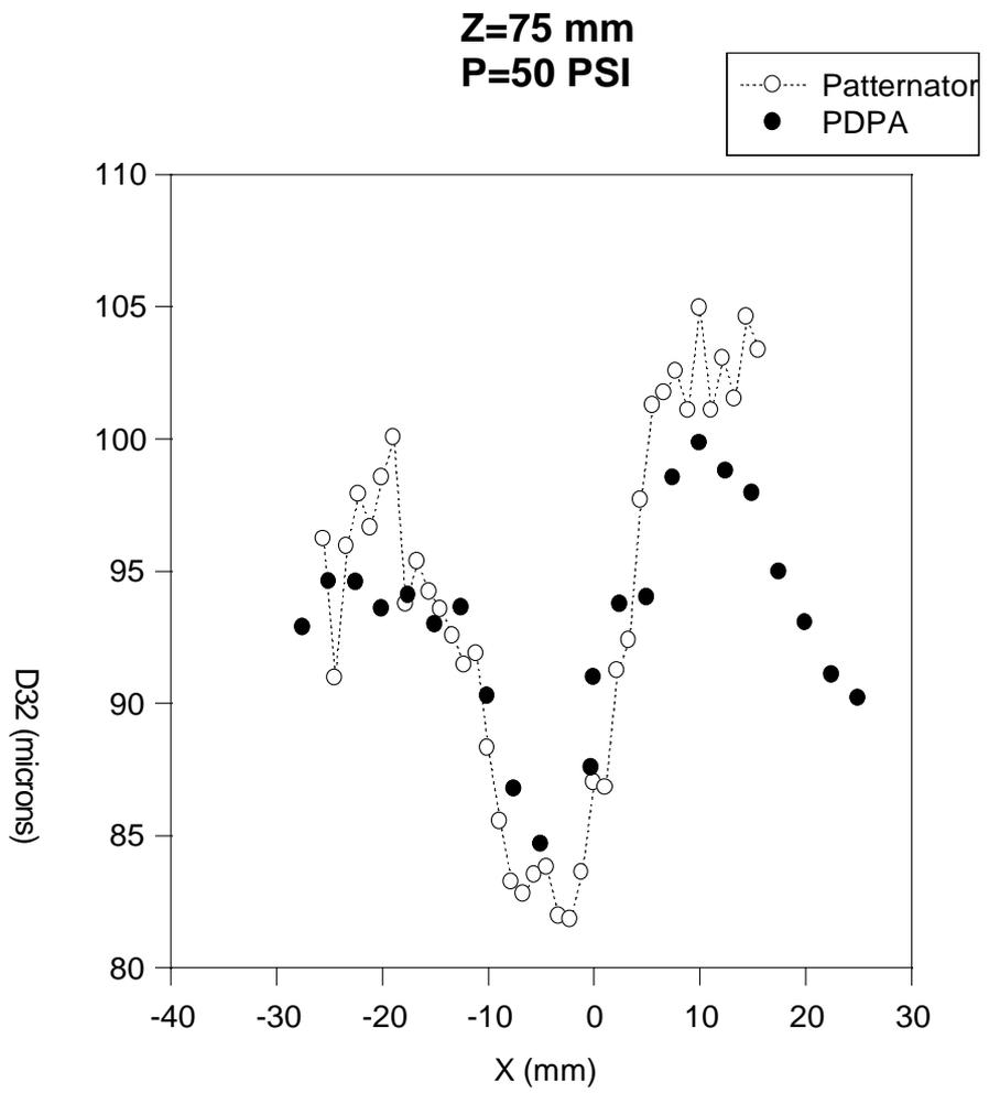
*Radial variation of the SMD at an axial location Z=75 mm. Comparisons of PDS and PDPA measurements, W.D. Bachalo 1994.*
