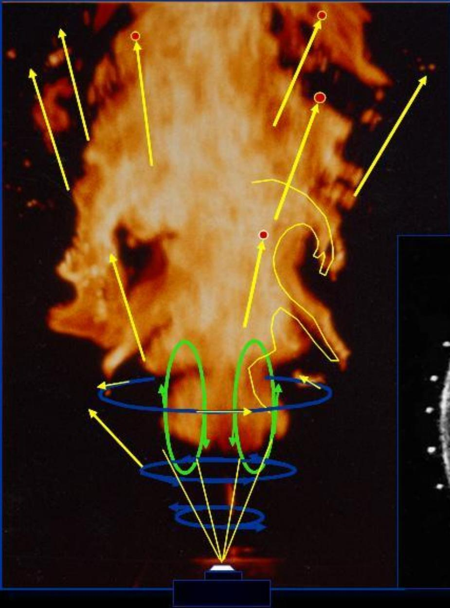
**Understanding the point measurement response of particle clusters passing the sample volume (Eulerian reference frame).**
