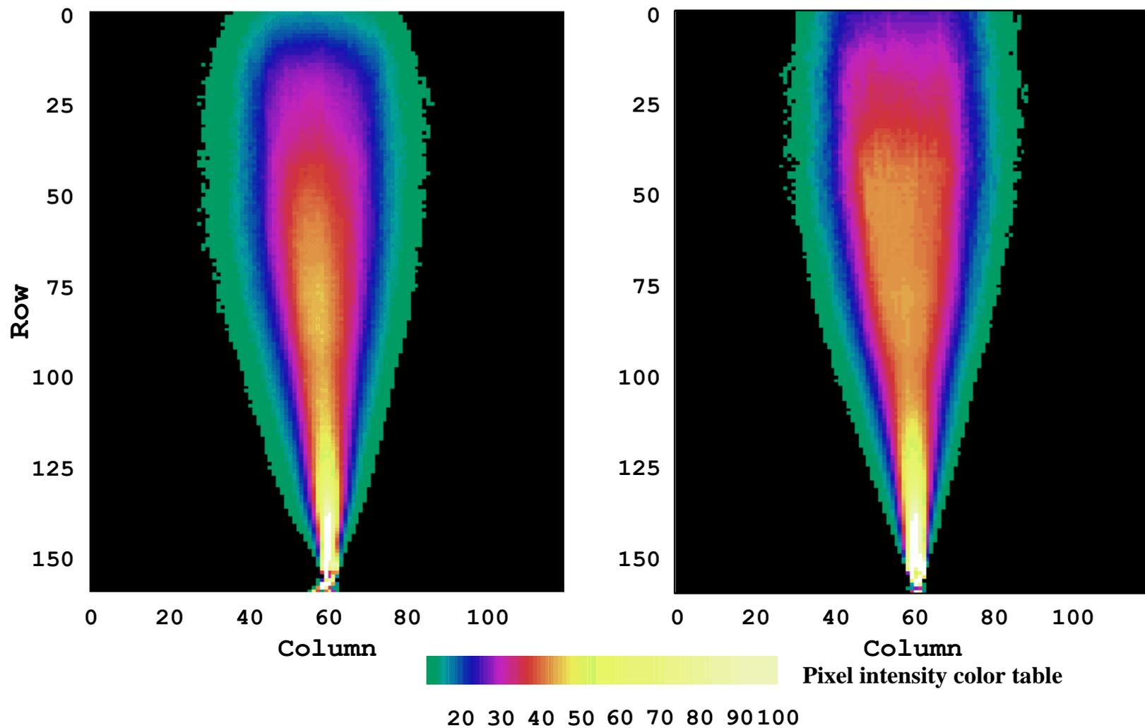
*Fluorescence and Mie Scattering images of the spray used to obtain  $D_{32}$ ,*
