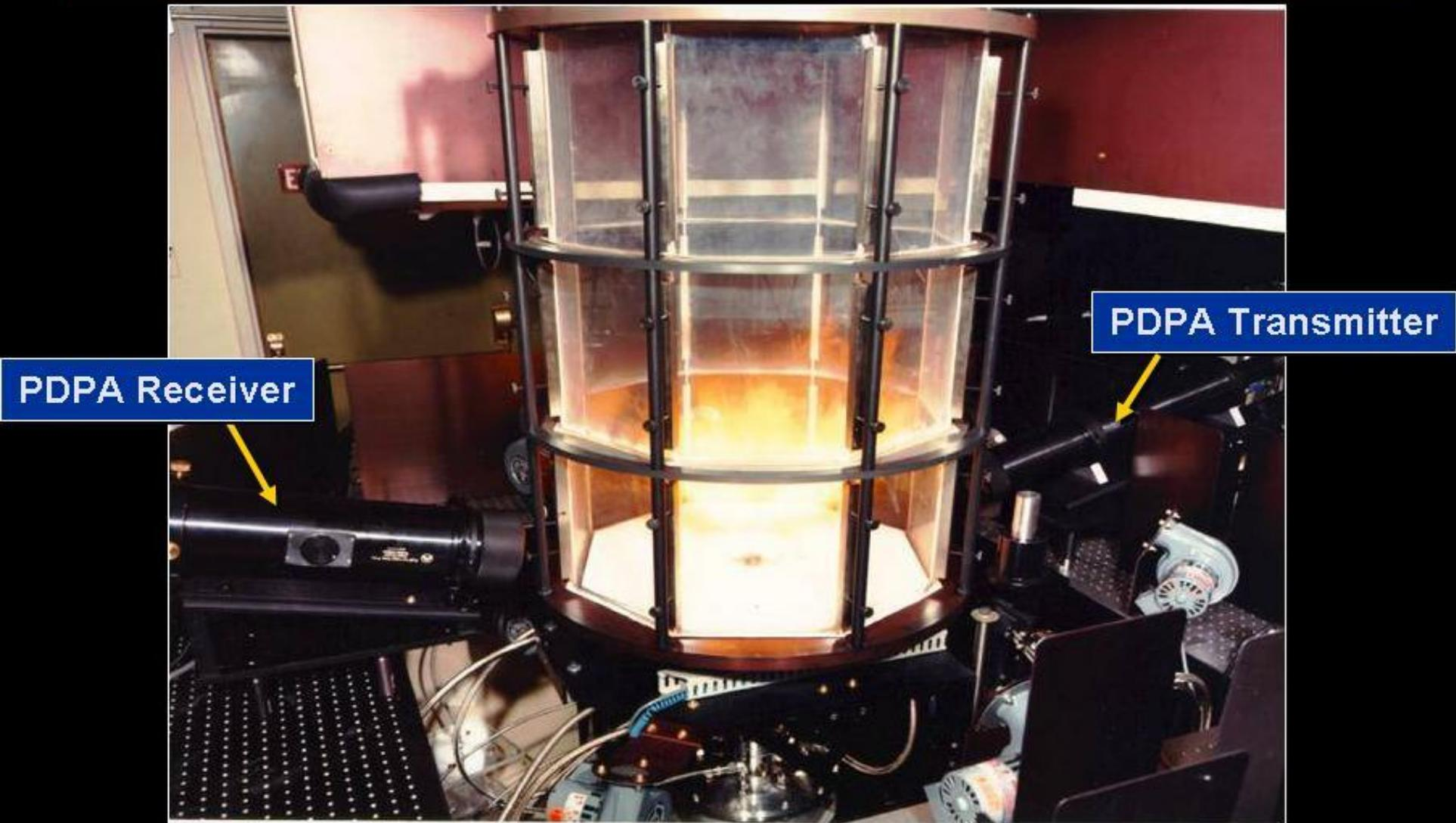
*Spray flame measurements at Sandia National Laboratories using an Aerometrics PDPA, C. Edwards, R. Rudoff, and W.D. Bachalo 1990.*
